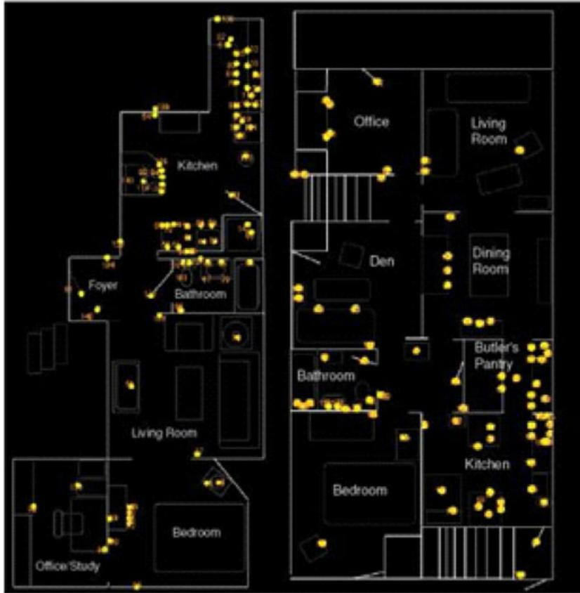
Figure 3. Location for placement of sensors in two homes [60].
